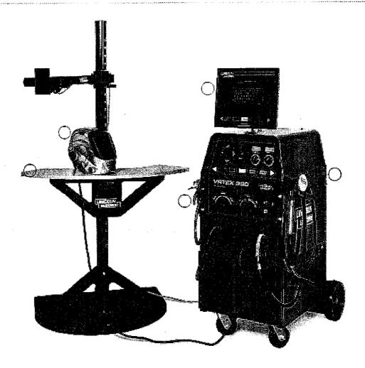
The VRTEX® is an educational training tool that is designed to accelerate welding training through the utilization of virtual reality. Use the VRTEX® System to simulate:
